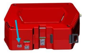
To do this, press the Factory Default button <u>before</u> the boot process and hold it down for approx. 10 seconds during the boot process. The PWR LED flashes rapidly when the device is reset to factory settings. As soon as the PWR LED lights up continuously, the web interface is accessible again.
