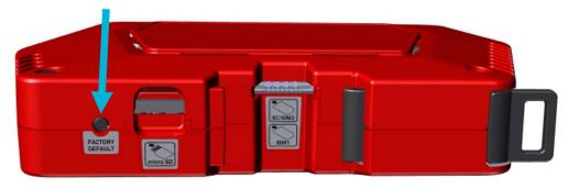
The Factory Default button must be pressed <u>prior</u> to the boot-up process and held down for approx. 10 seconds during the boot-up process. The PWR LED flashes rapidly while resetting to factory settings. As soon as the PWR LED illuminates constantly, it is possible to access the web interface.
