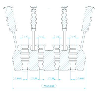
Type 2: 3 x hole 5...7 mm; 1 x hole 3...5 mm
