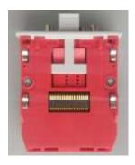
Insert the module so that the contacts point towards the circuit board.
