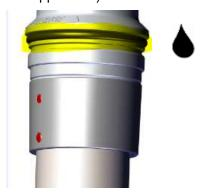
13. Slide on the sealing sleeve:
