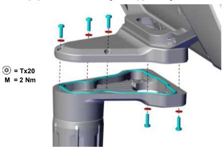
4. Screw the Key module to the flange below.
