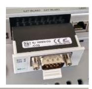
Lower the module approx. 5 mm from the edge of the housing so that the metal brackets come to rest in the recesses in the circuit board.
