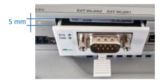
Then, **lift the module a bit** to lift the metal brackets out of the circuit board.
