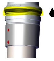
13. Slide on the sealing sleeve:
