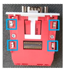
The metal brackets must be inserted into the **recesses** in the circuit board:
