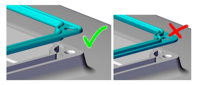
Press in the seal **at the corners first**. Then press in **evenly** along each edge from the outside to the inside in order to avoid rippling.
