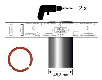
The screws included in the scope of delivery may be used for fastening (hexagon head screws similar to DIN 6921 M5x10 and M5x16).
