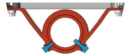
Here, a screw presses on a blind hole in the tube. Another screw sits in a through hole in the tube. Both screws have a polyamide coating on the thread.
