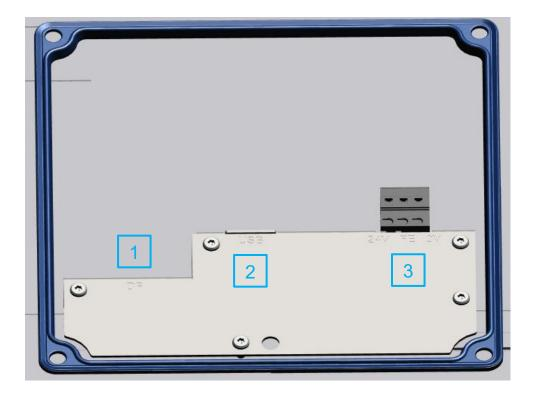
Display port – or – HDMI for transmitting the image signal
